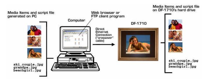
Figure 1: Direct Connection to One DF-1710
