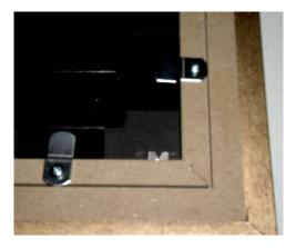
8) Adjust the four black frame brackets in their slots so that they are snug against the inner surface of the offset clips on the frame (this compensates for the varying notch depth of different frames and varying mat and glass thicknesses) and re-tighten the machine screws holding the brackets to the DF-1710.
