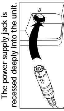
Be sure that the arrow on the connector is aligned with the arrow on the Digi-Frame case.
